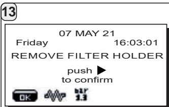
13 At the end of wash cycle, the message "REMOVE GROUP FILTER HOLDER" will appear.
